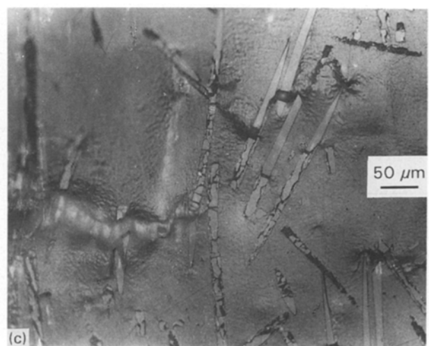
Figure 18 In situ fracture observations of 30 wt % glass composite showing (a) higher degree of matrix plasticity in the crack front, (b) formation of deformation zone by connecting the plasticity region at fibre ends, and (c) limited crack bridging by glass fibres in the crack wake.
